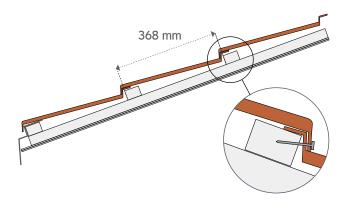
The panels are placed onto battens spacing 368 mm. The downturned front edge and the upturned rear edge of each tile provides a strong, weatherproof, overlapping and interlocking roof covering. Each panel is secured by 4 nails in the front downturned edge into the side of the batten, positioned out of the water course.
